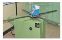
Vertical Load Balancing Machine
